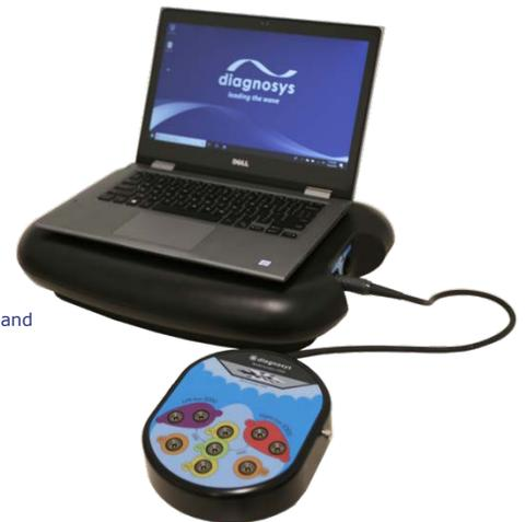
E<sup>3</sup> console, 32-bit amplifier, computer and Espion software.
